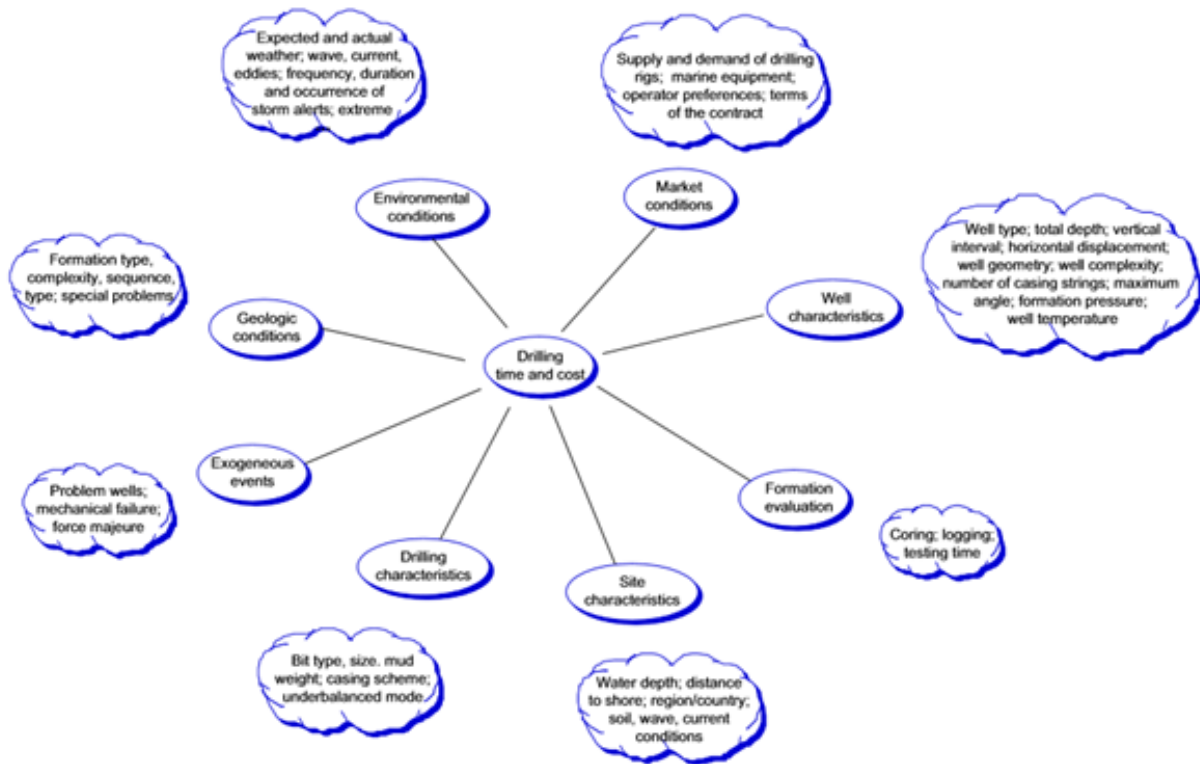
Fig 3.8 : The time and cost to drill a well is influenced by a number of variations
