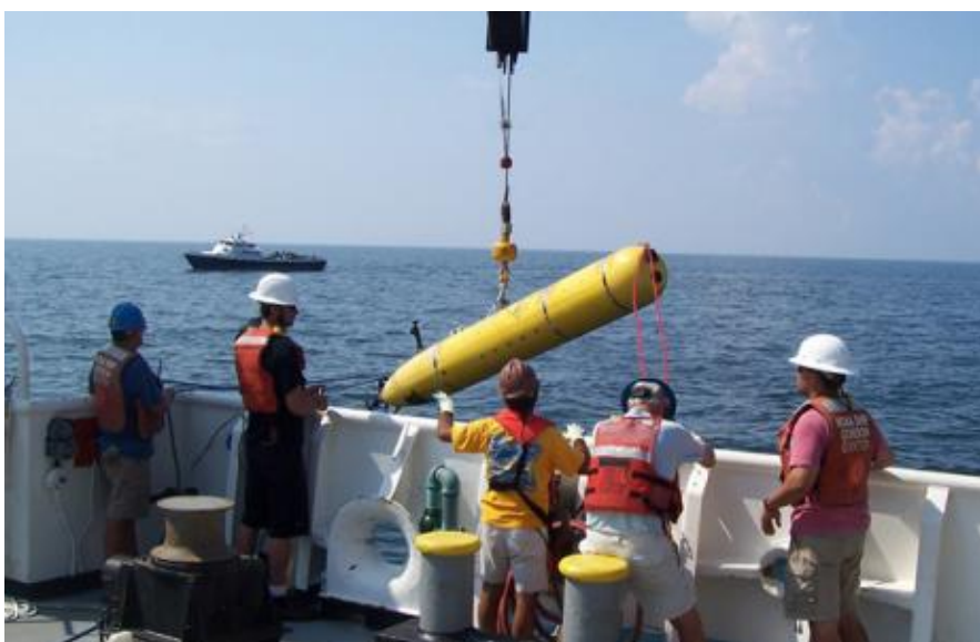
Fig 10.13: Yanwu Zhang 2010 MBARI, An autonomous underwater vehicle from the Monterey Bay Aquarium Research Institute (MBARI) being launched from the NOAA Ship Gordon Gunter in the Gulf of Mexico.
