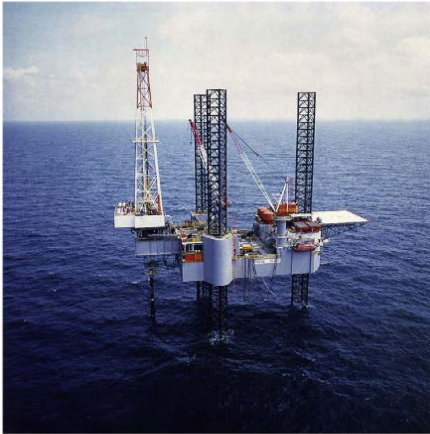
Fig. 3.12. Mobile offshore drilling unit – jackup. Source: Pride.
