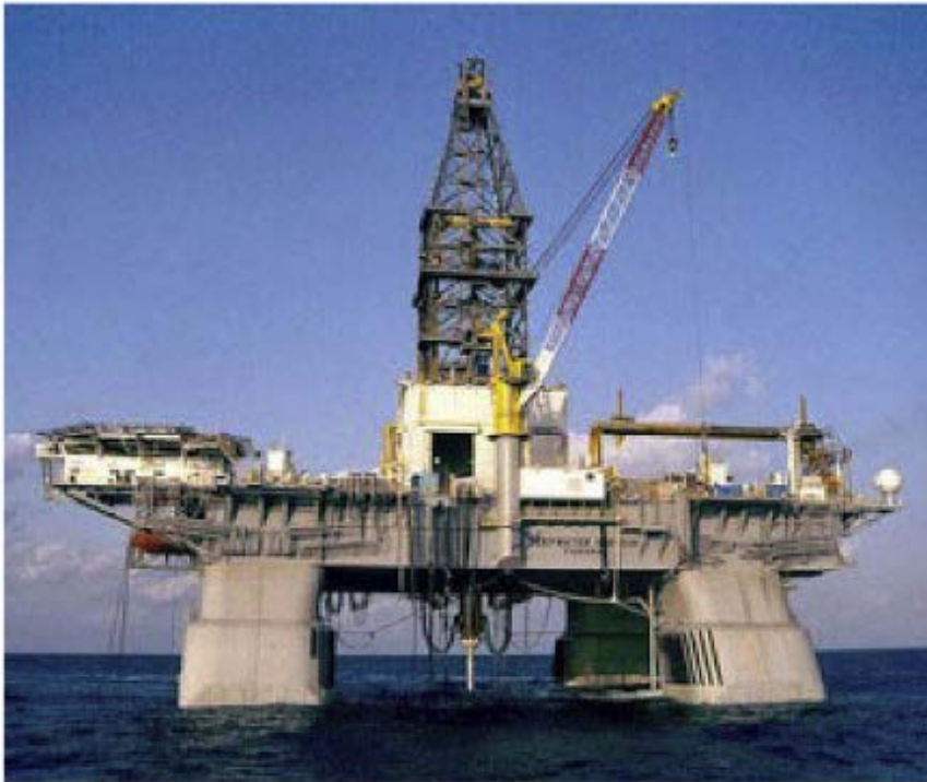
Fig. 3.13 Mobile offshore drilling unit – semisubmersible. Source: Transocean.
