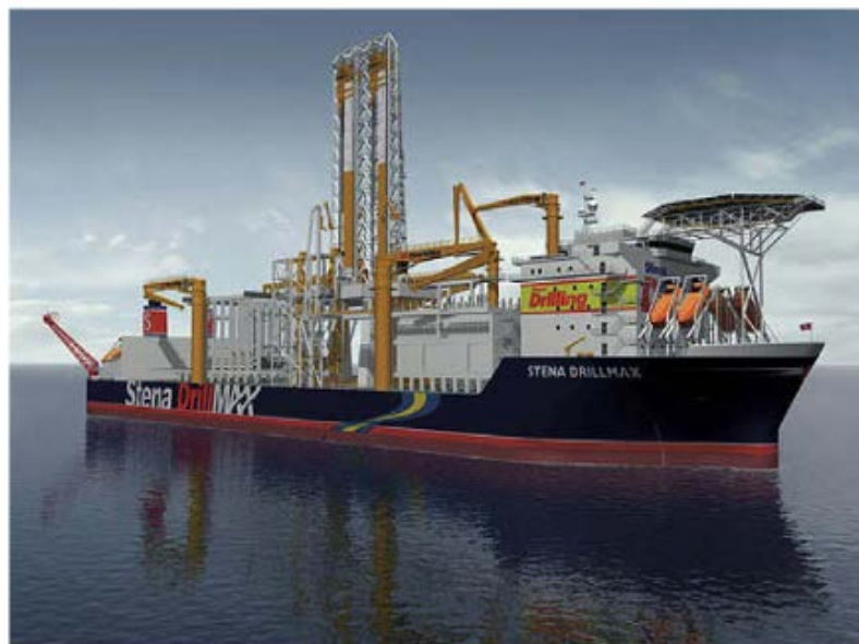
Fig. 3.14. Mobile offshore drilling unit – drillship. Source: Stena Drilling
