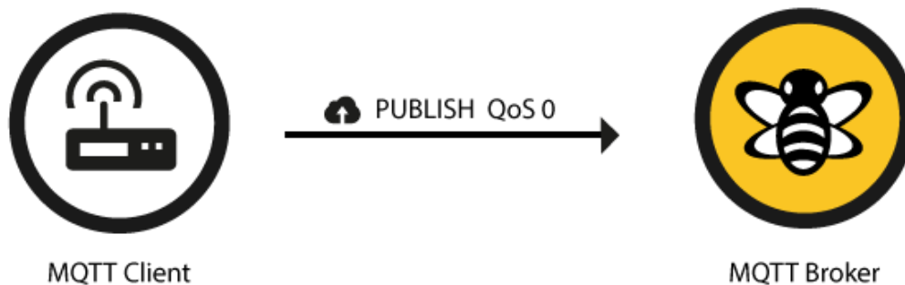
Figure 2: MQTT Quality of Service 0. [5]
