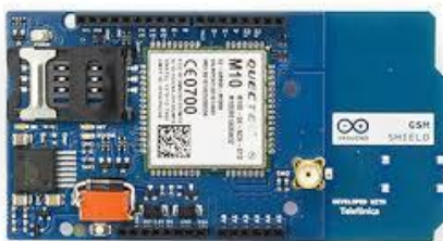
Figure 15: Arduino GSM shield
