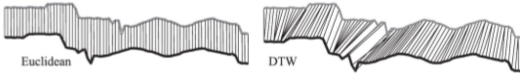
Figure 2.5: The mapping of a trajectory using either the Euclidean or the DTW function [42]
