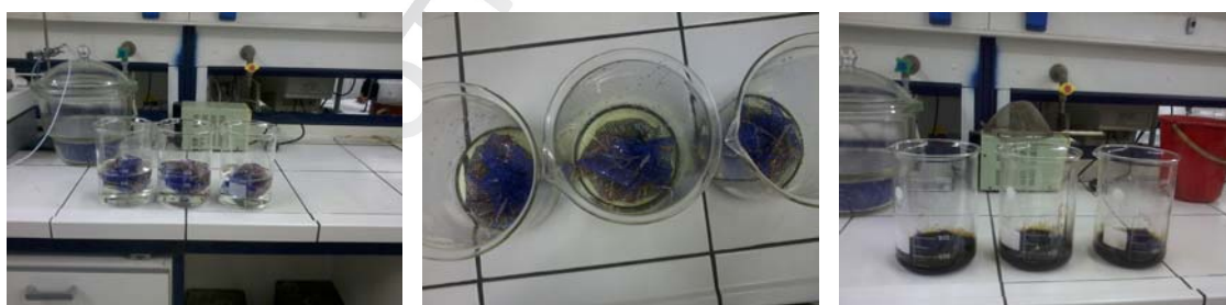
Fig. 10.2 Packed AWS-II in the case of pure liquids experiments; water (left), diesel (middle) and crude oil (right)
