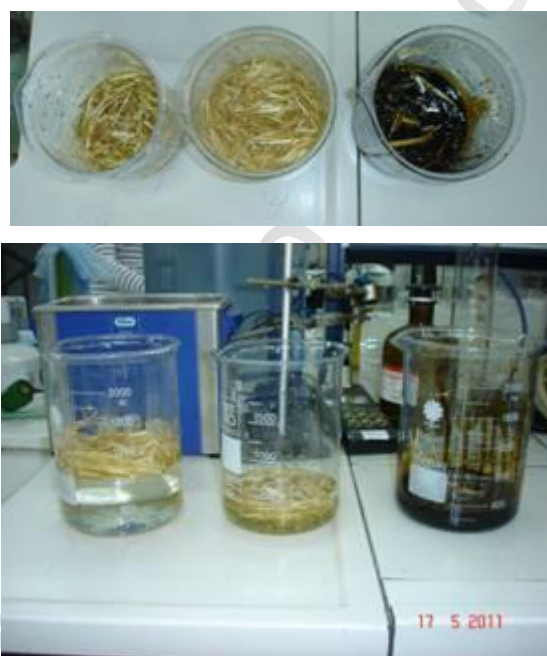
Fig. 7.3 Water (left), Diesel oil (middle) and Crude oil (right) adsorbency testing experiments according to ASTM F 726-2012 method
