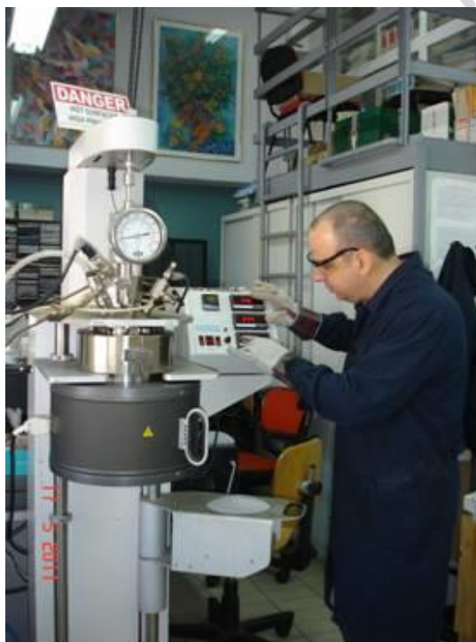
Fig. 7.1 The 3.75-L batch reactor PARR 4843
