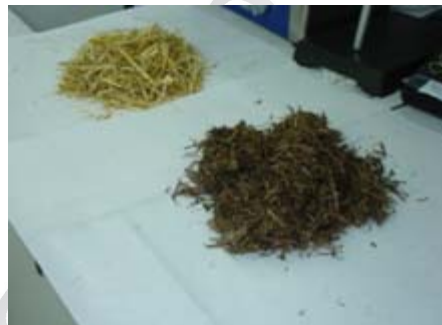
Fig. 8.5 Untreated (up left) and pretreated by acid hydrolysis (down right) barley straw
