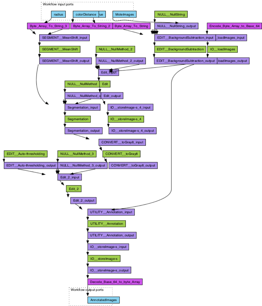
Figure 112. Workflow of the proposed approach for detecting and annotating the lesion areas from skin cancer images.
