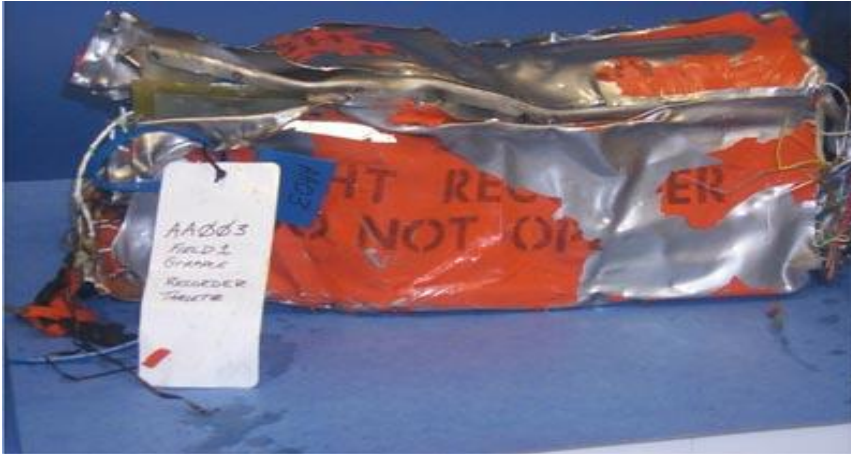
Εικ.39: The damaged flight data recorder from EgyptAir Flight 990
