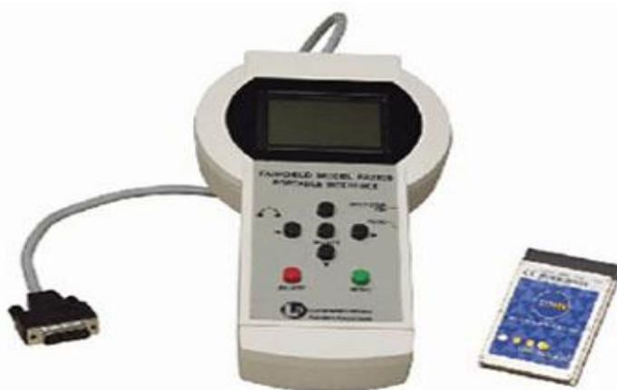
Εικ.43: This portable interface can allow investigators quick access to the data on a black box.
