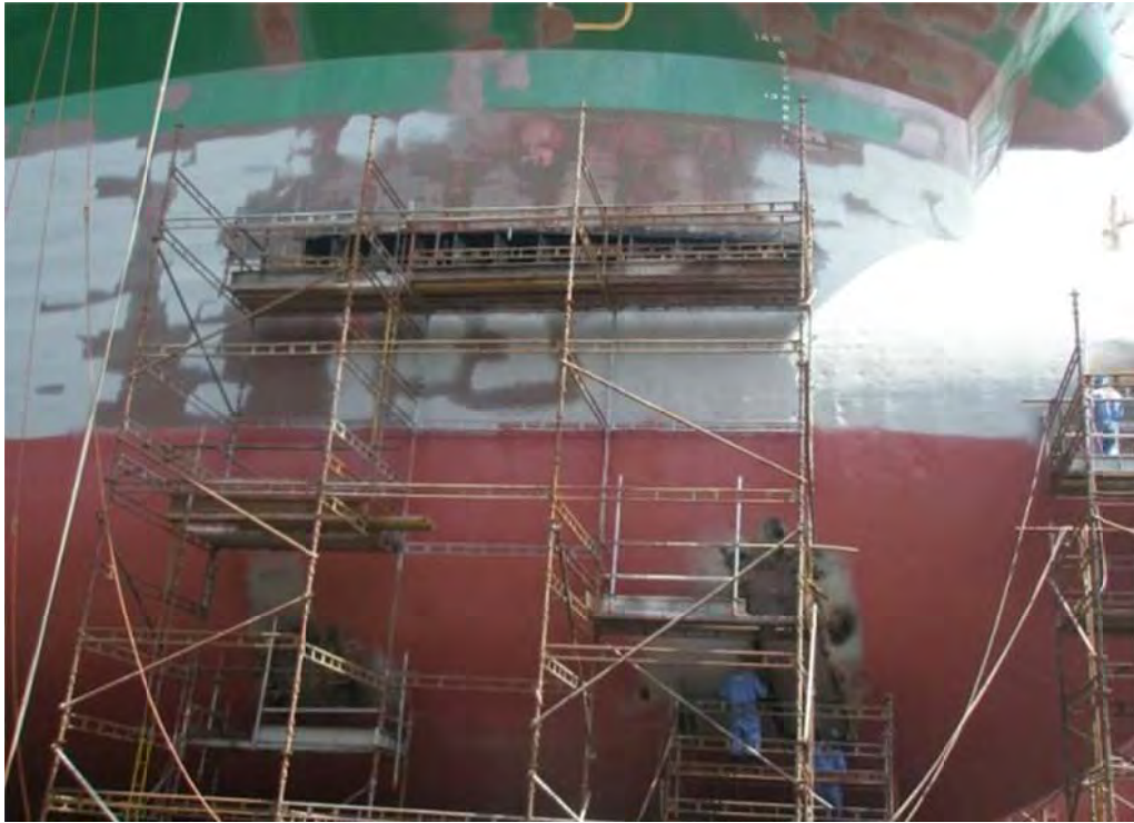
Picture 21: Side shell steel repair
