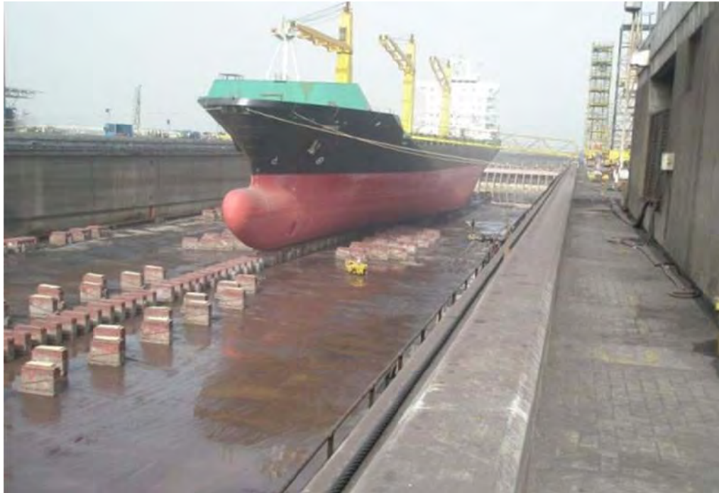
Picture 9: Container ship resting on keel blocks
