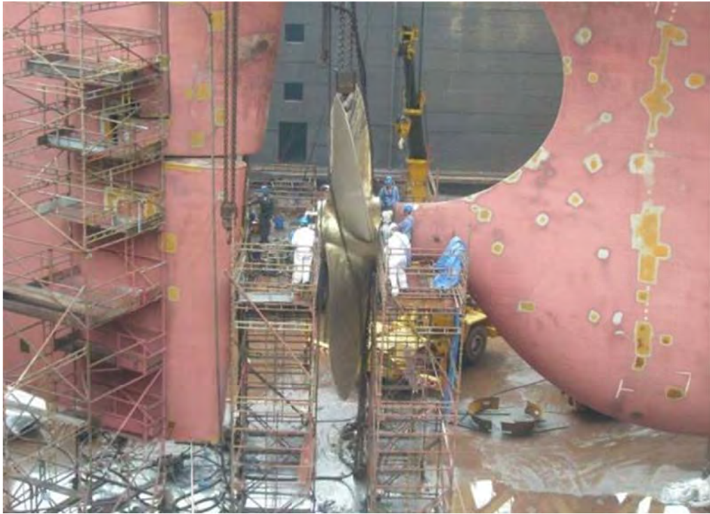
Picture 11: Propeller removal in a dry-dock
