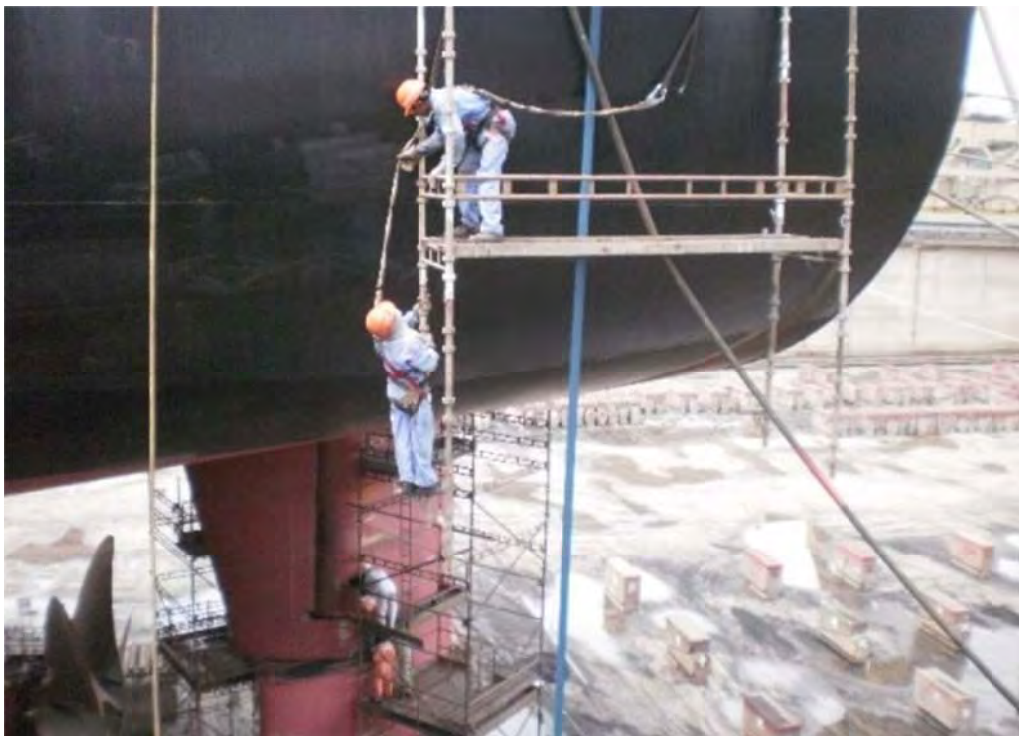
Picture 26: Erecting hanging staging
