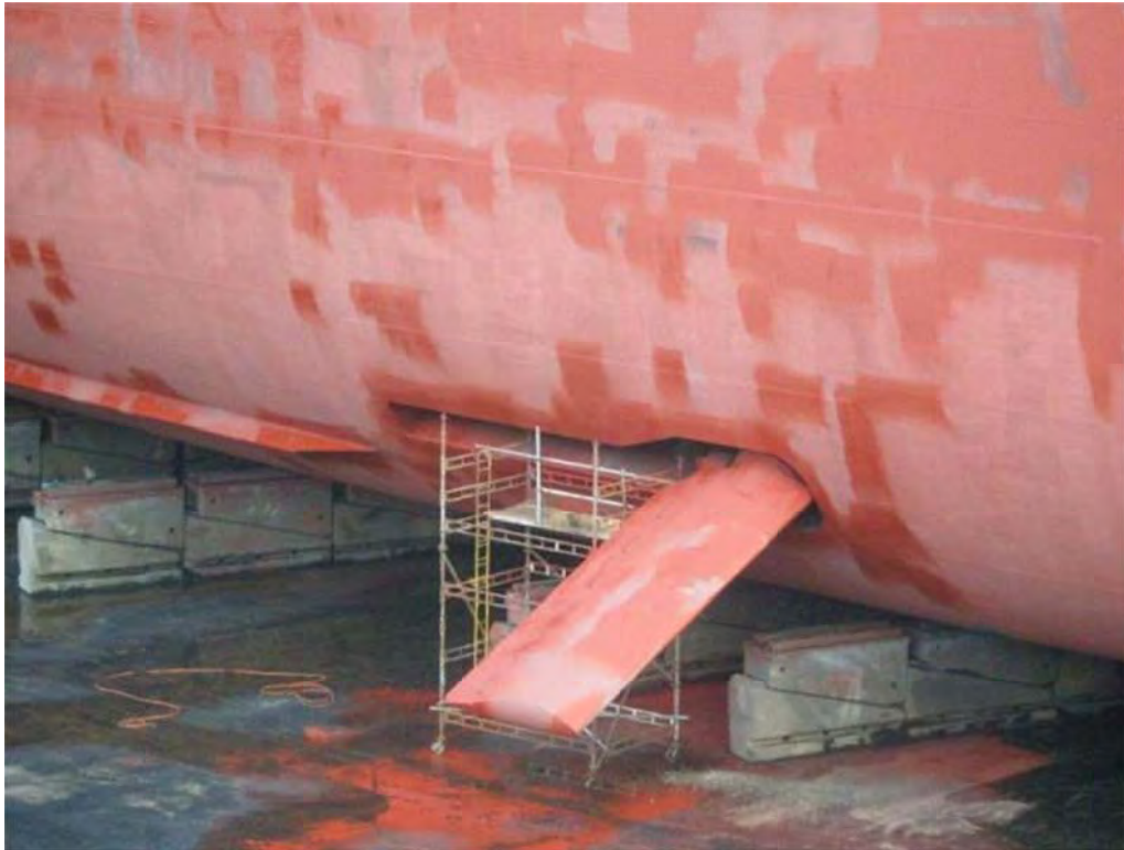
Picture 14: Inspection of stabilising fins
