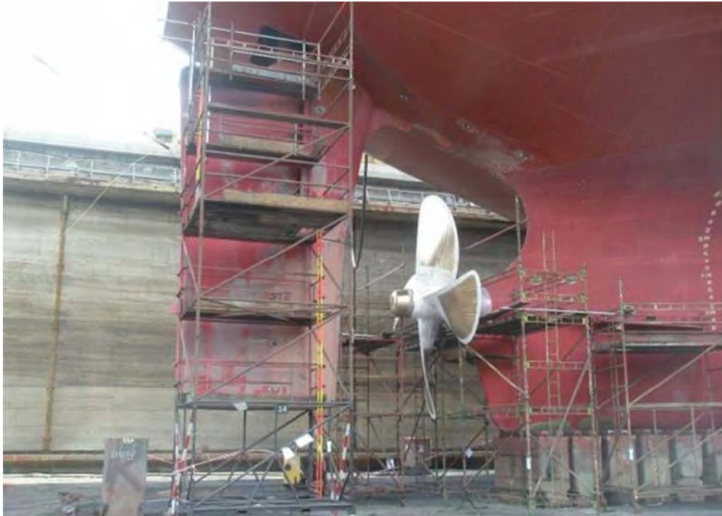
Picture 13: Polishing and dye-checking of propeller
