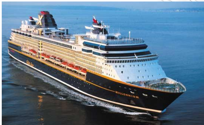
Σχ. 6-1: Cruise Ship “MILLENNIUM”, LOA = 294m, B = 32,2m, 2xGELM 2500+
