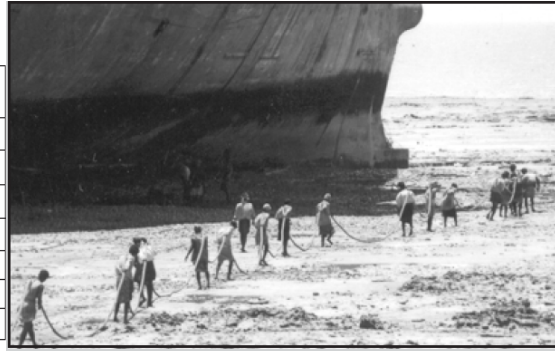
Photograph 5 : Labour of wire group are pulling wire on shoulders.
