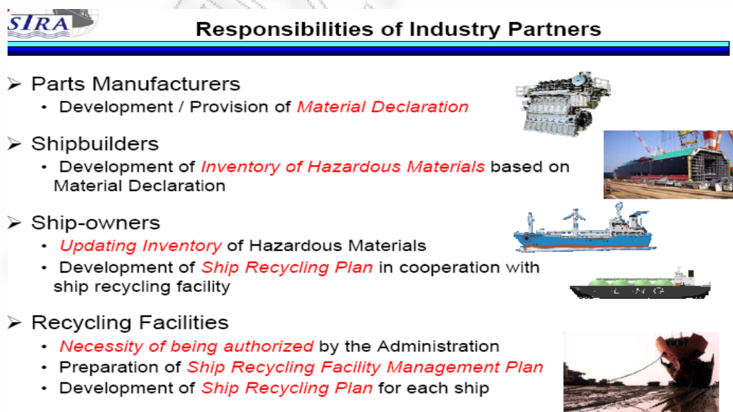
Figure: Responsibilities of Industry Partners – Source: Ship Recycling Convention - What does it require shipbuilders to do? - Tasuku Hirabara, Japan Ship Technology Research Association
