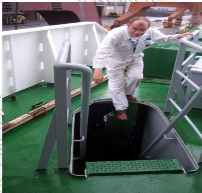
lack of any safety railing
