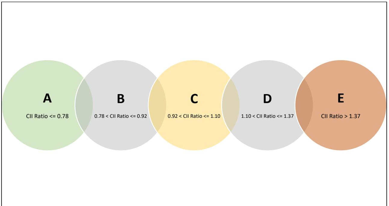
Figure 20: CII Rating based on CII Ratio for LNG Carriers with DWT  $< 100,000$
