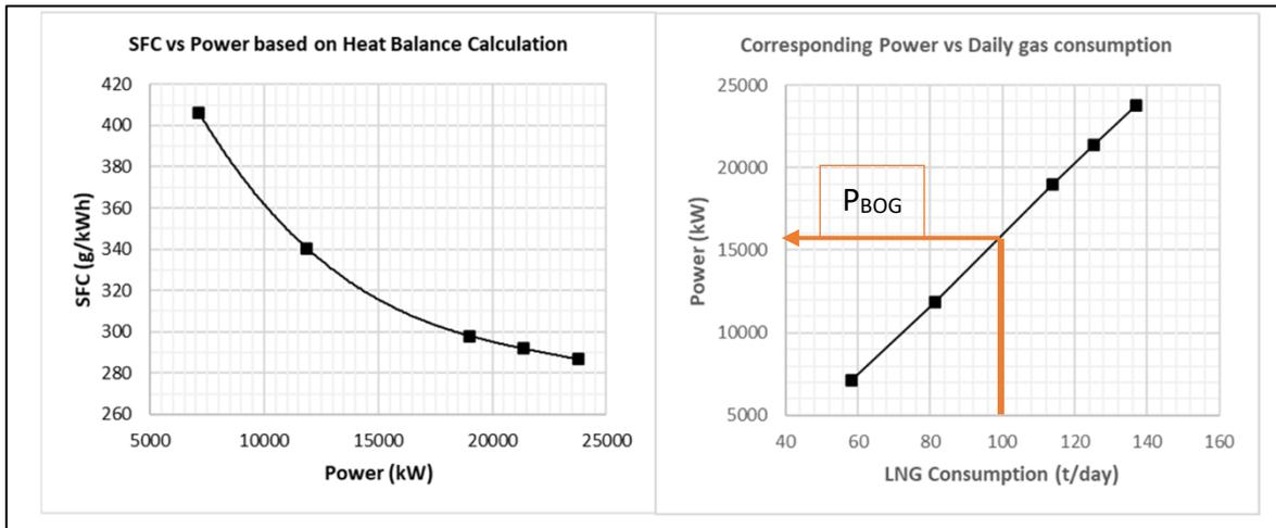
Figure 16: Example of SFC vs Power from Heat Balance and Corresponding Power vs Daily LNG Consumption for a typical LNG Steam Turbine Ship [22]
