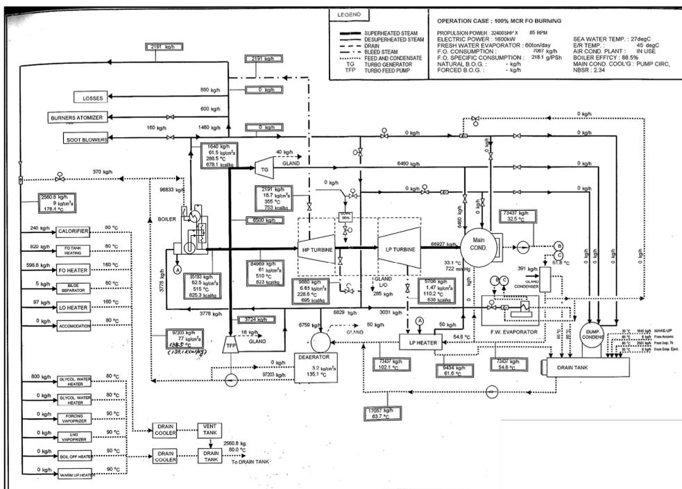
Figure 7: Indicative operation of steam boiler plant at 100%<sup>1</sup>
