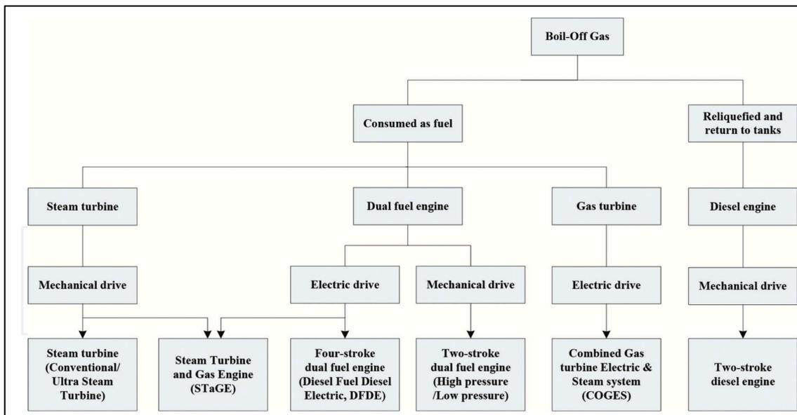
Figure 4: Categorization of propulsion systems for LNG carriers [5]
