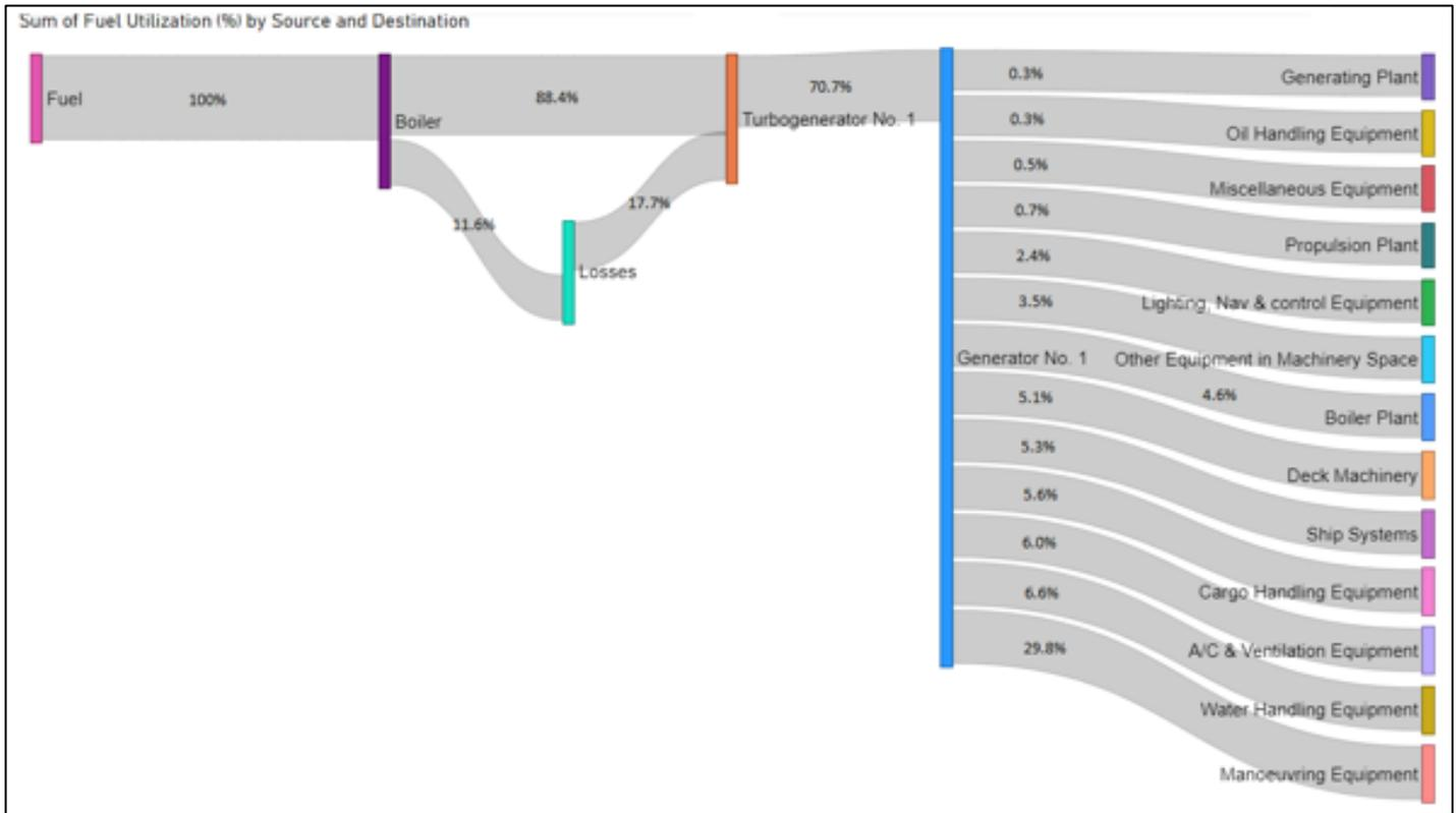
Figure 26: Fuel Utilization Percentages and Energy Flow at Port Condition
