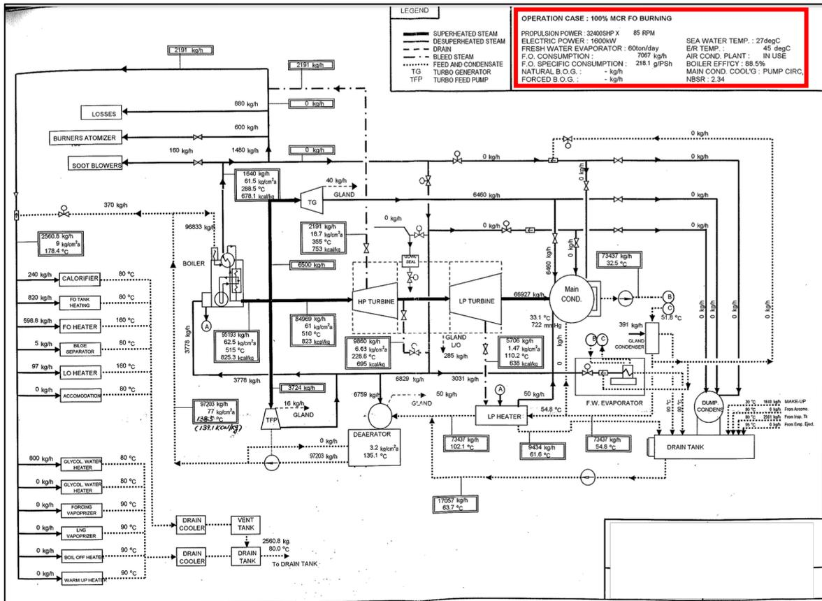
Figure 30: Indicative Steam Heat Balance and Flow Diagram
