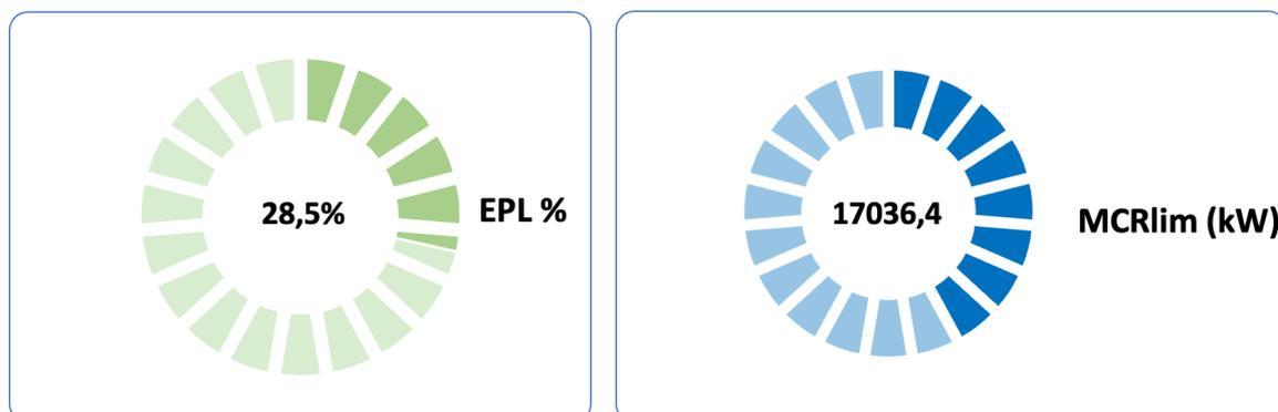
Figure 21: EEXI Results of Ship A
