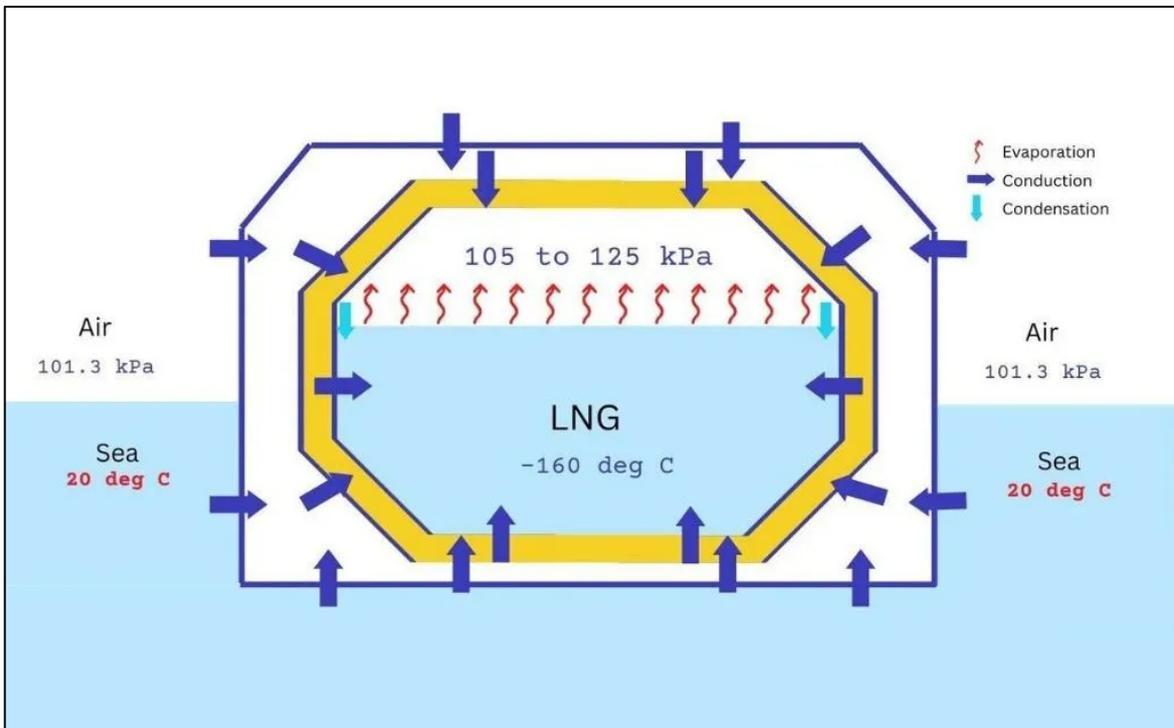
Figure 15: Boil-off Gas on LNG prismatic tank [21]
