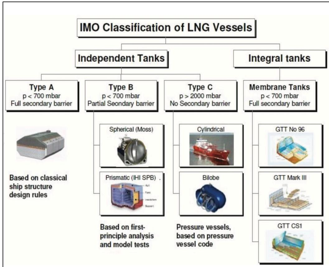
Figure 3: Categorization of containment systems for LNG Carriers.[5]
