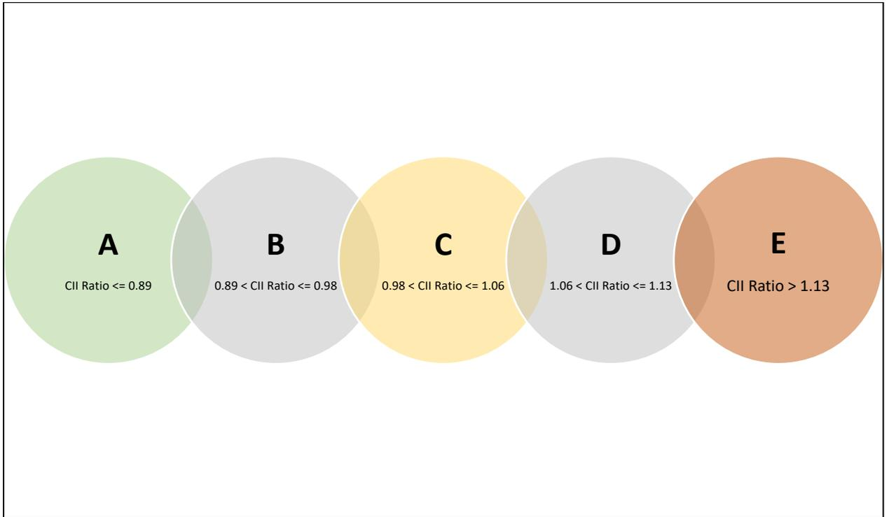
Figure 19: CII Rating based on CII Ratio for LNG Carriers with DWT  $\geq 100,000$
