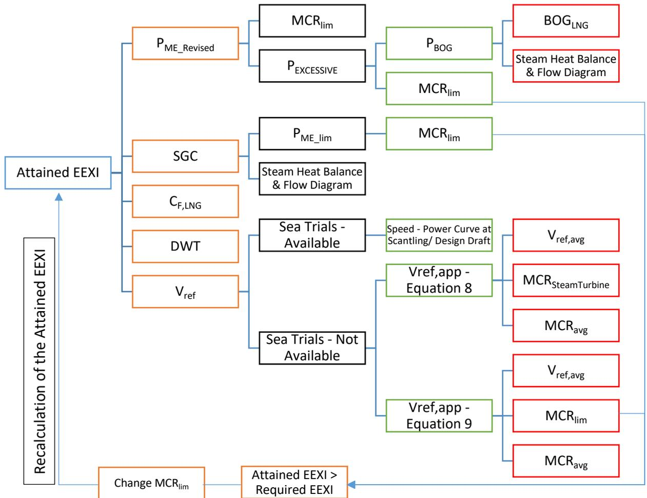
Figure 17: Flow Chart for the calculation of the Attained EEXI for LNG Steam Turbine vessels
