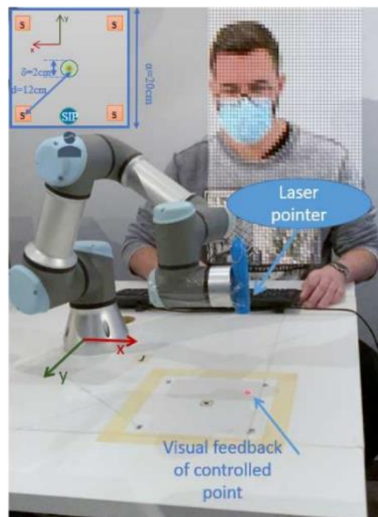
Figure 2.7: Human-Robot Collaboration setup [30]. The robot's movements are onstrained within a 20cm \times 20cm area - a schematic representation of the area is presented in the upper left corner of the figure. The EE is placed in one of the four starting ('S') positions and the HR team has to bring the EE in the centre (green area) of the square. A laser pointer attached to the EE of the robot provides to the human visual feedback about the position of the EE that is controlled.
