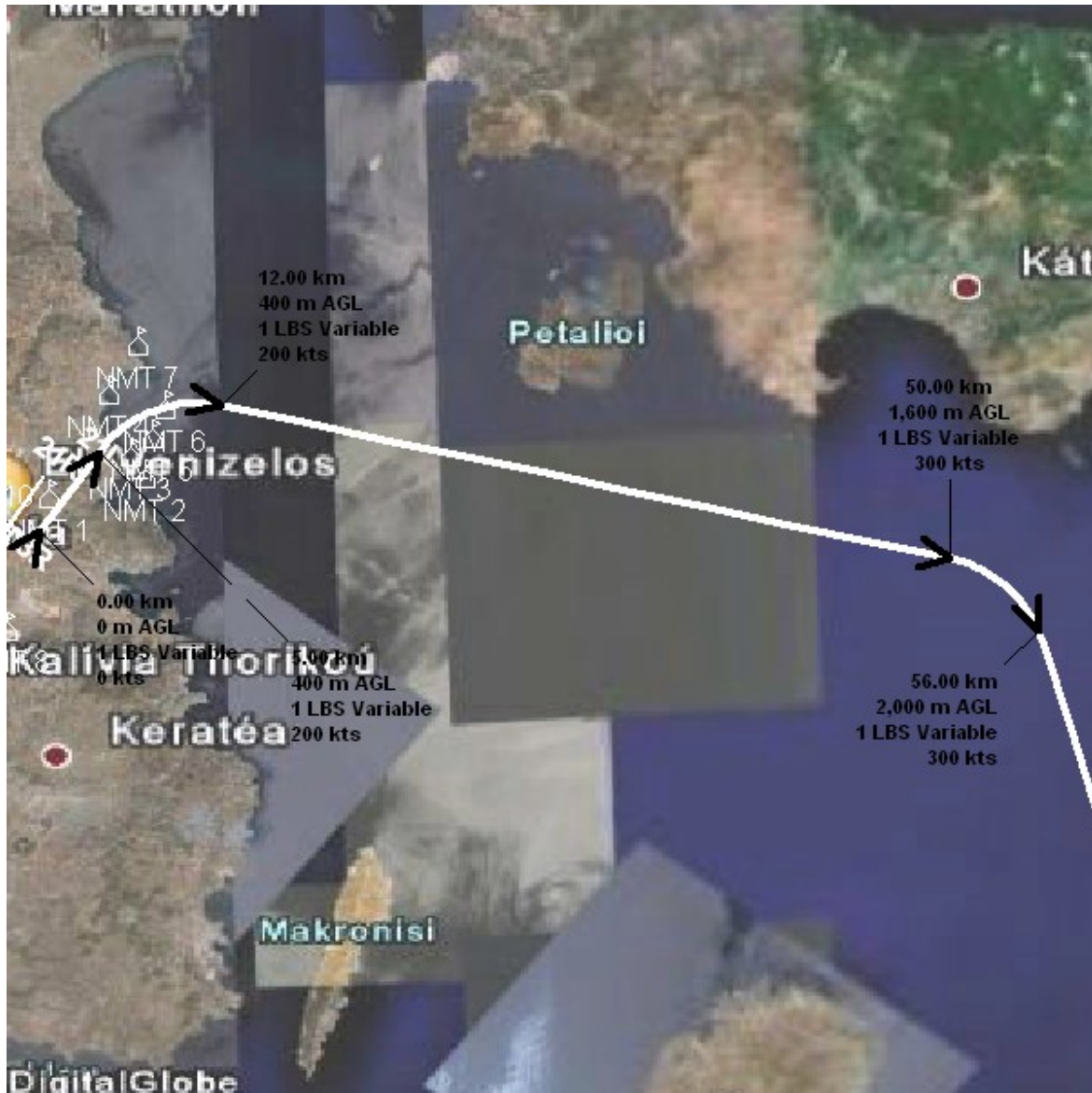
Flight Profile VARIX 1JA3 Flight Track: VARIX 1J Aircraft: Based A320* Engine: CFM56-5A-1 0 20,000 40,000 40,000 80,000 100,000 Scale in Feet
