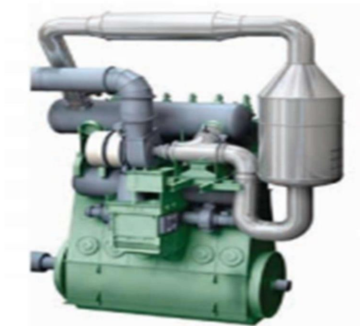
Picture No.1: Scrubber system in a 2-X engine (Source – Kirtatos, 2010)
