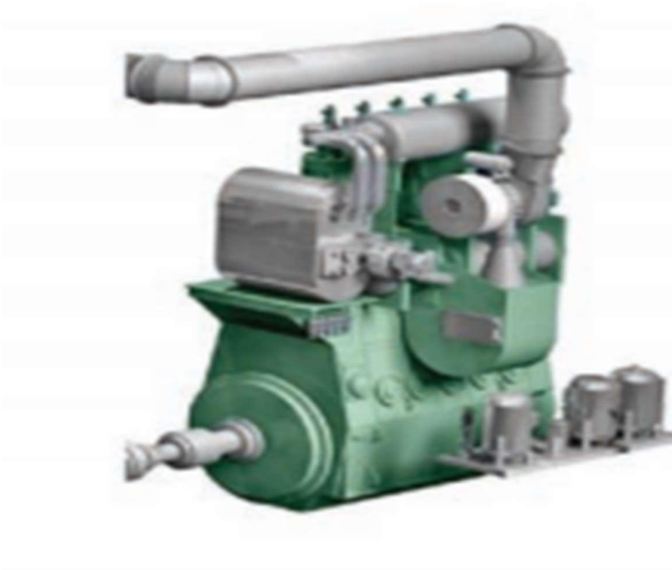
Picture No.2 - Exhaust gas feedback system - EGR in 2-X engine - (Source: Kyratos, 2010)
