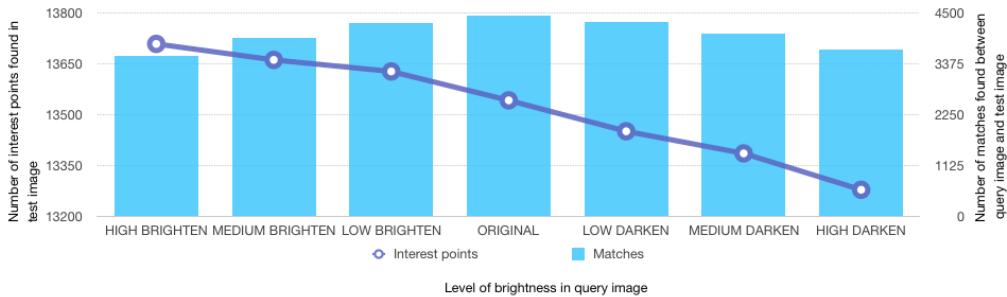
Figure 58 – Graphical representation of matches found between query image and test image and interest points found in test image as the brightness changes.
