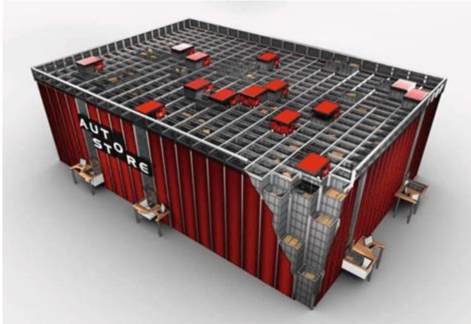
EΙΚΟΝΑ 29: ROBOTIC CUBE STORAGE ( https://www.beer-management.de/cube-storage-systems-market-overview/ )
