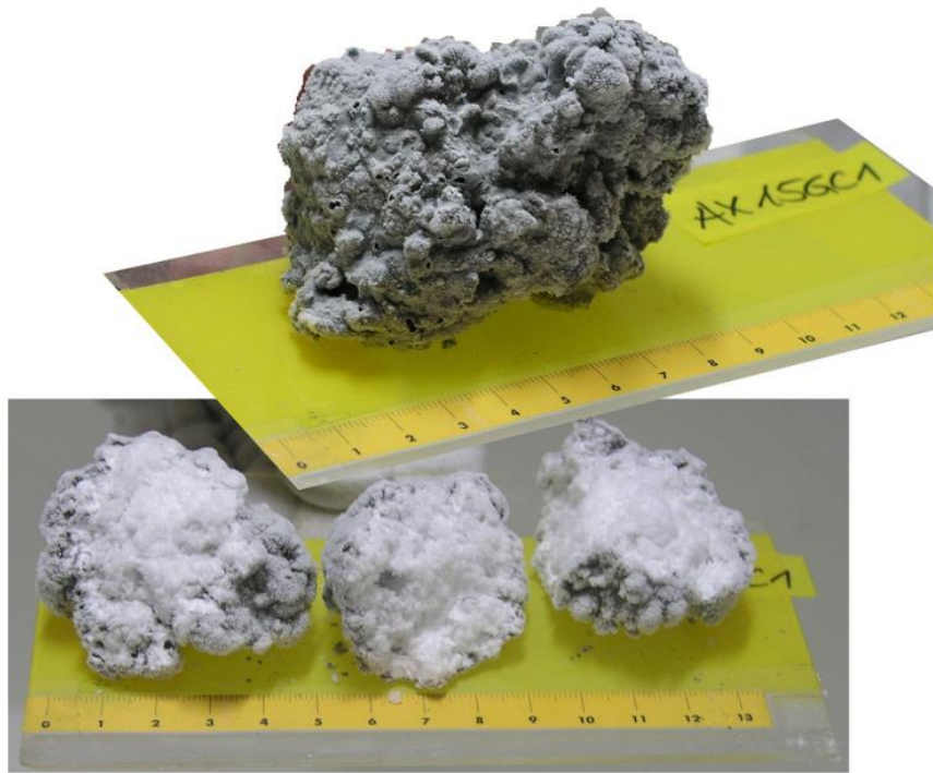
Figure 22: Gas hydrate lump (8 _ 5 _ 4 cm) (center) and broken into pieces (lower) that was recovered from one of the cores from Amsterdam mud volcano . (Lykousis et al., 2008) .
