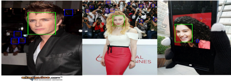
Figure 15: Example of false predicted bounding boxes.
