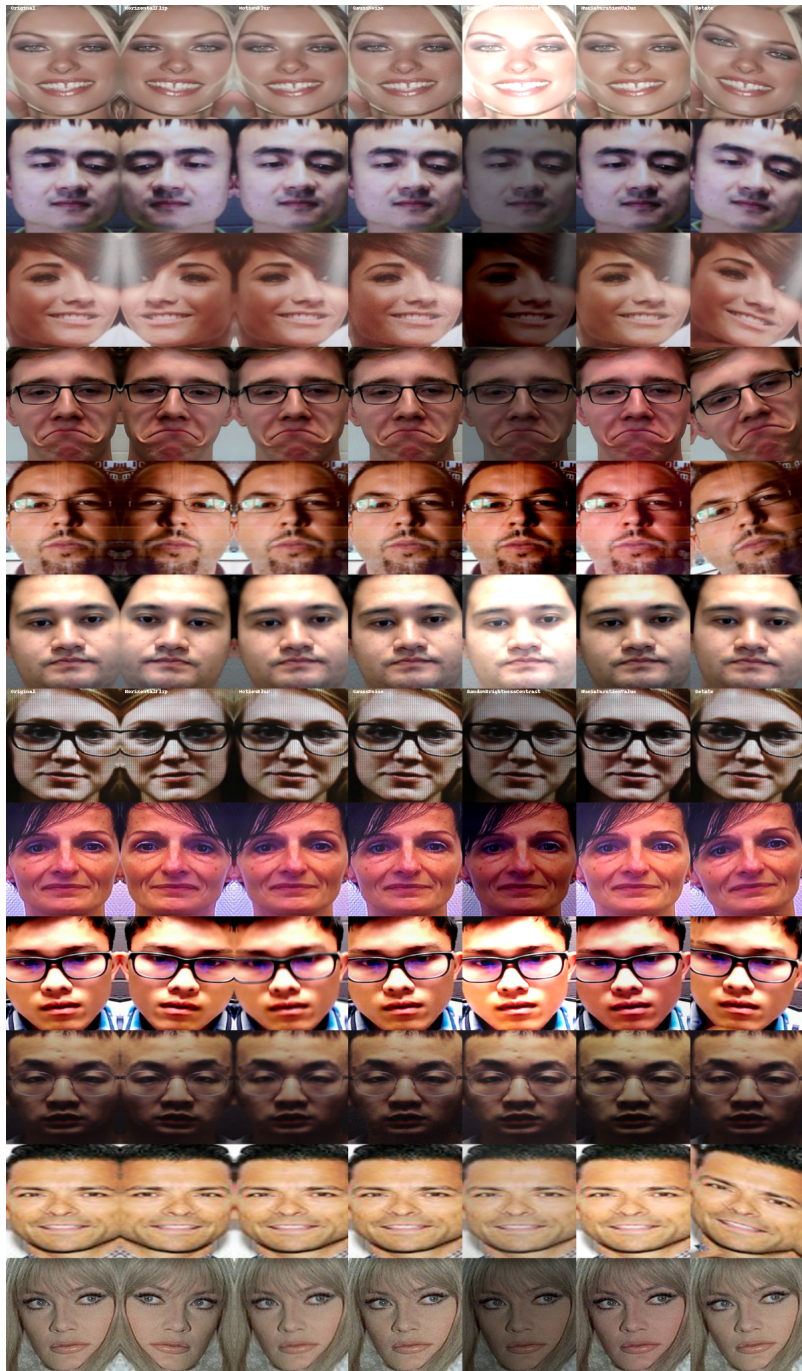
Figure 26: Augmentations with the following order Original - HorizontalFlip - MotionBlur - GaussNoise - RandomBrightnessContrast - HueSaturationValue - Rotate
