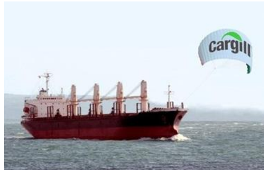
Image 8 The largest kite-powered ship.
