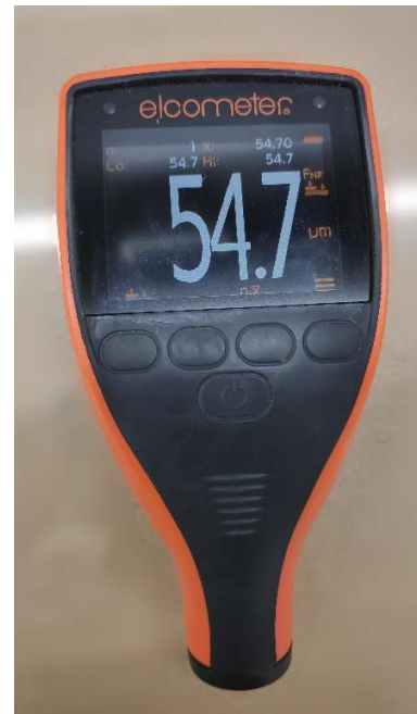
Figure 18: Elcometer 415 for DFT measurement
