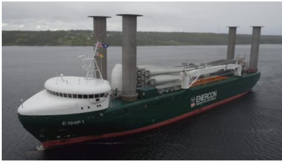
Figure 8.3 Chemical ship with 4 flettner rotos on deck
