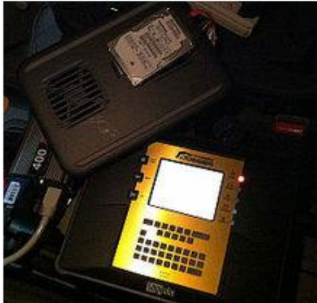
Figure 4: Imaging a hard drive in the field for forensic examination.
