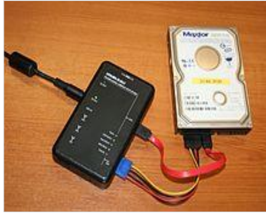
Figure 1: A portable Tableau write-blocker attached to a hard drive.
