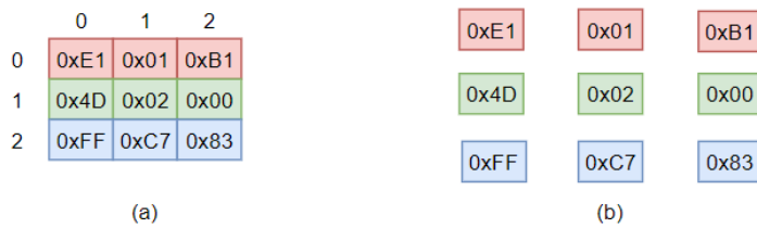
Figure 20. ARRAY_PARTITION Complete example (a) Two-dimensional array, (b) Partitioning for d=0
