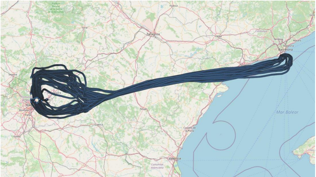
Figure 34. Barcelona to Madrid Gail Results with behavioral cloning for pre-training with expert trajectories enriched with NOAA and METAR.
