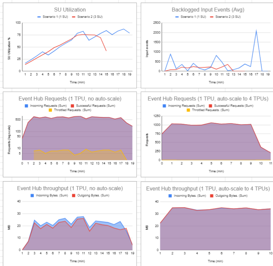
Figure 4-4: Visualizations of throughput, requests, SU utilization and backlogged event metrics for both scenarios.
