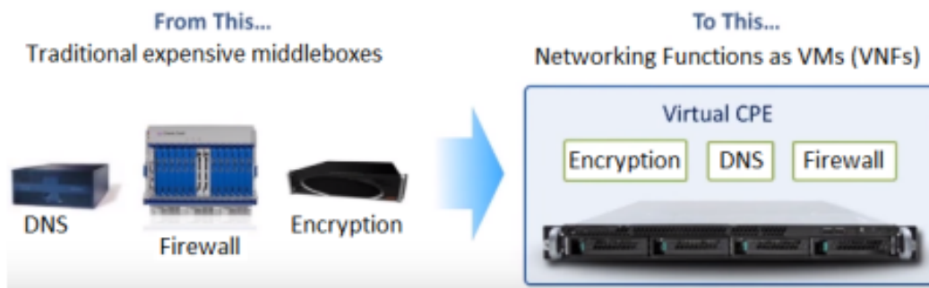
Figure 1: Network Function Virtualization
