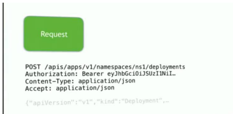
Figure 24 - Example of an API request with a bearer token and how it is parsed
