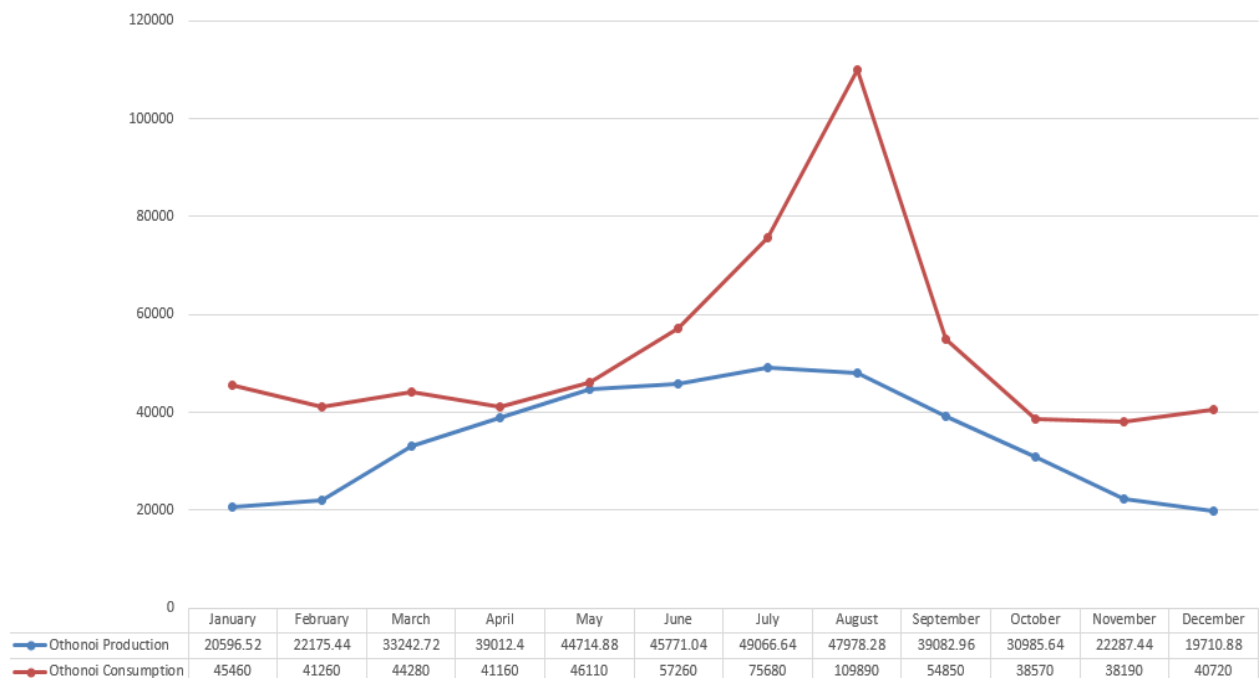
Figure 26: Energy consumption in kWh (red) in the island of Othonoi. PV generation in kWh (blue) per month under the proposed scheme.
