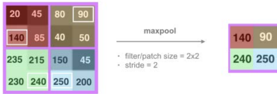
Figure 11 A maxpooling layer reduces the x-y size of an input (output of the activation function) and only keeps the most active pixel values.
