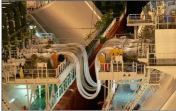
Εικόνα 5.3.4.1 ship to ship transfer with flexible hoses
