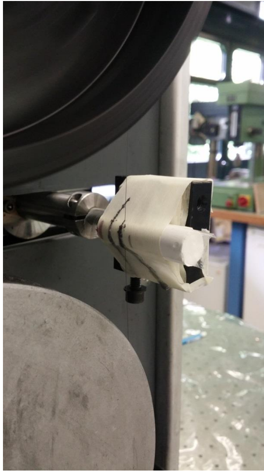
Fig. 3.4 : Performed cut in a cylindrical CPC specimen using diamond wire saw.
