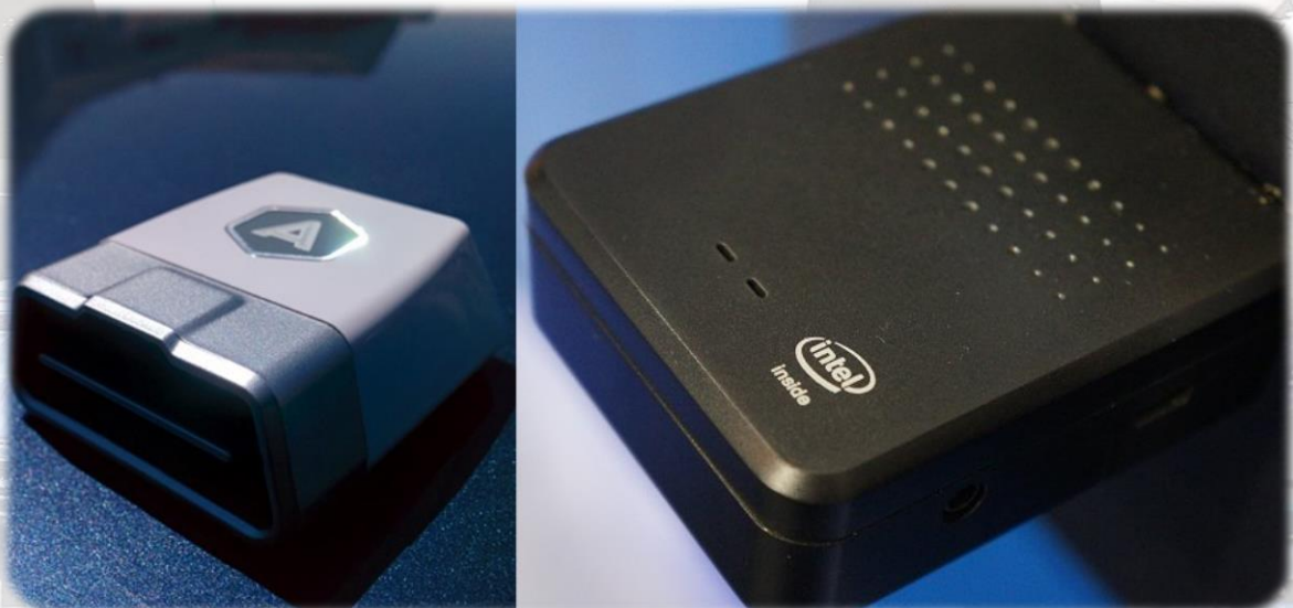
Image 10: AutomaticLink (left) and Intel on board diagnostics units, compatible with legacy vehicles, through the dedicated DIN slots ( hardwarezone.com , 2016) 12
