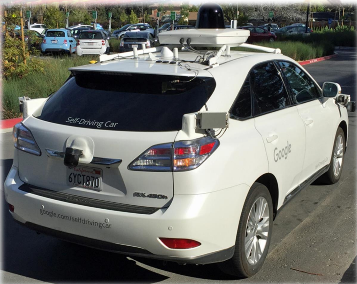
Image 14: Lexus RX 450h, one of Google's self-driving vehicles, used in digital "capturing" of highway and urban routes around regions, enhancing Google Maps with the recent Street View feature ( forbes.com , 2016) 16
