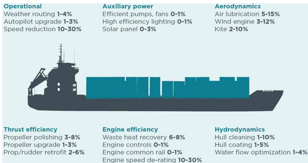
Figure 1: Potential fuel use and CO 2 reductions from various efficiency approaches for ships (International Council on Clean Transportation (ICCT), July 2013). Long-term potential for increased shipping efficiency through the adoption of industry-leading practices.
