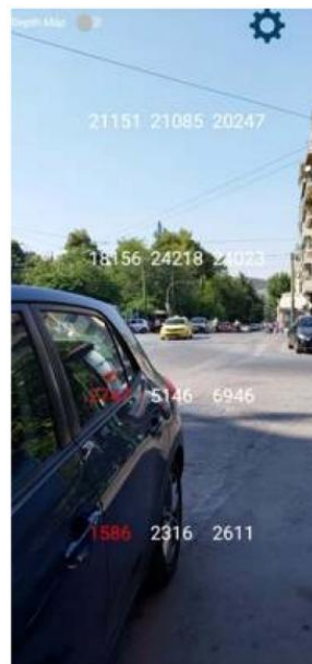
Figure 47: Example showing the system successfully identifying the parked car using Low Bound metric of 4500. The parked car is identified at the bottom left side of the grid, where cells are highlighted with red color.
