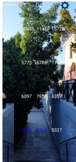
Figure 49: Example showing the system successfully identifying the stairs going down. Stairs are identified at the bottom left side of the grid with distance labels highlighted with blue.
