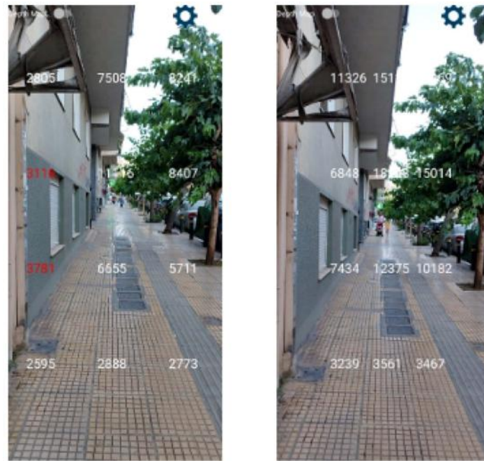
Figure 50: The initial example (Left) wrongly indicates obstacles on the far left of the scene while the final version (Right), which uses the 60% of the width, indicates no obstacles. Obstacles are identified where the distances are highlighted with red color.
