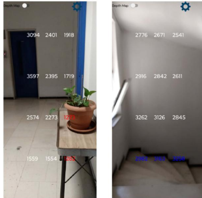
Figure 40: Execution of the system in indoor area. On the left, the obstacle is identified successfully with lights on (distances highlighted with red), while on the right, the stairs are identified successfully, with lights off (distances highlighted with blue).
