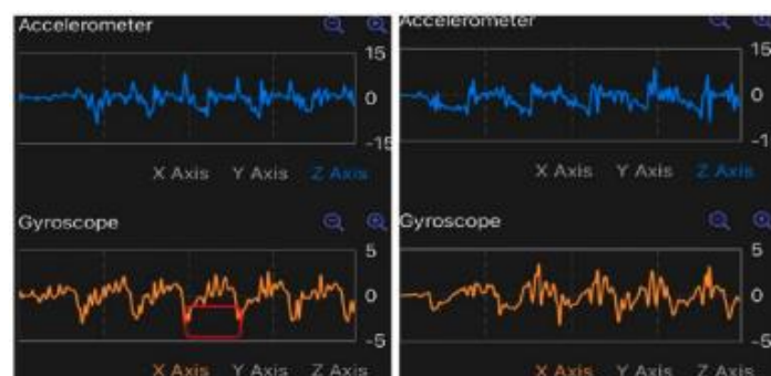
Figure 29: Results from the paretic right leg scenario of the system. The red box indicates a full gait event.
