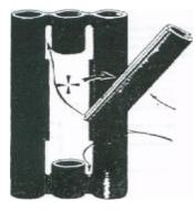
Damaged tube à Saw horizontally through the tube where marked at top and bottom keeping as level as possible. Remove tube with the membrane fin attached. Remove membrane fin from both sides of tube and one side of adjacent fin 2 "above cut and" below at top and 2" and 1" at the bottom. File exposed ends of tube where the membrane fin was cut off so that it is made flush with the tube. Clean
