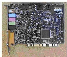
Fig. 3 - Sound card (Creative Labs SoundBlaster Live!)
