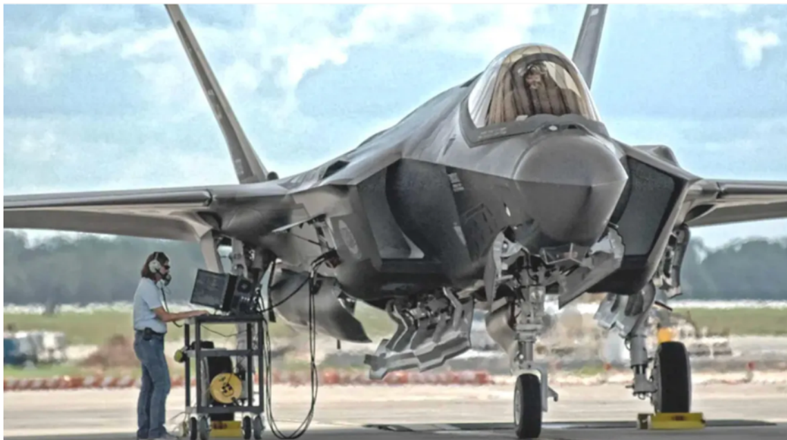
Picture 6. USAF F-35 Technician Downloading Data from Aircraft. (Credit: TWZ - https://twz.com )
