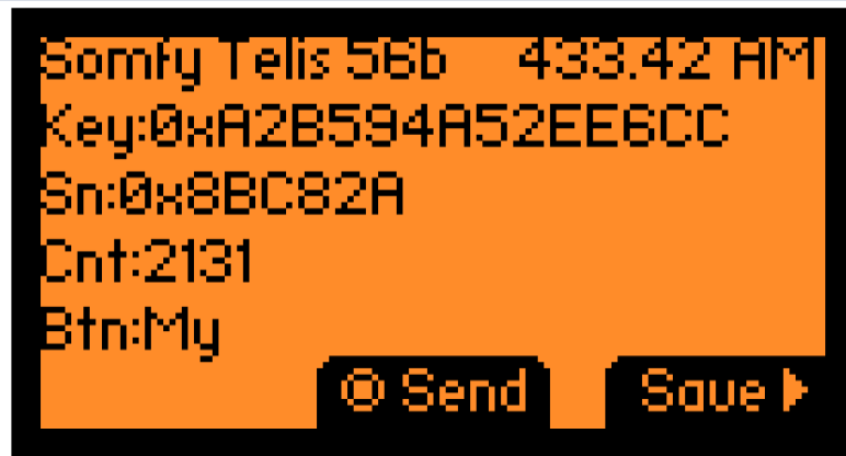
Figure 5.9: Breakdown of a Somfy RTS frame, showing the encryption key, the sender Serial Number (Sn: 0x8BC82A), and the rolling Counter (Cnt: 2131).
