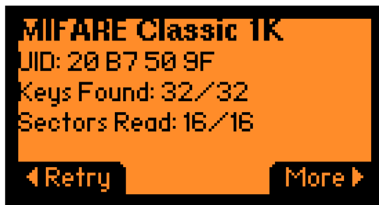
Figure 5.25: The dictionary attack recovering all 32 sector keys and reading all 16 sectors.
