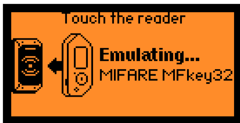
Figure 5.30: The key-extraction interface, which in a live attack would harvest authentication nonces from the physical reader.
