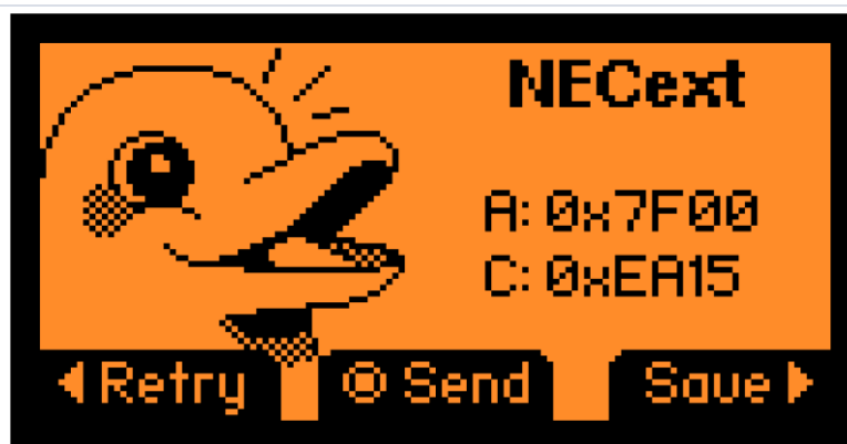
Figure 5.62: A captured TV "mute" command, decoded as the NEC-extended (NECext) protocol (Address 0x7F00, Command 0xEA15).
