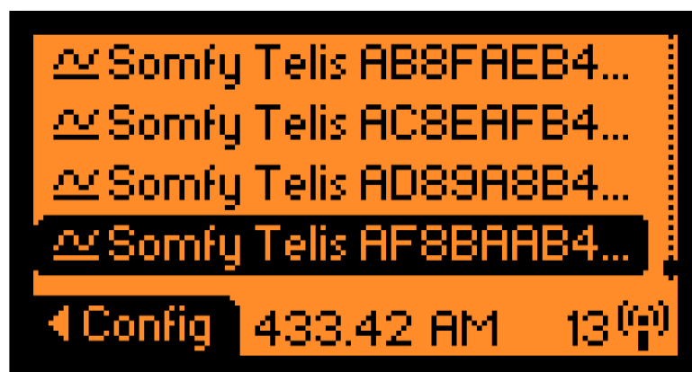
Figure 5.7: Passive interception of multiple Somfy Telis transmissions, each carrying a different payload.
