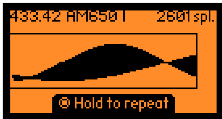
Figure 5.12: Continuous RAW playback producing sustained RF jamming on 433.42 MHz.
