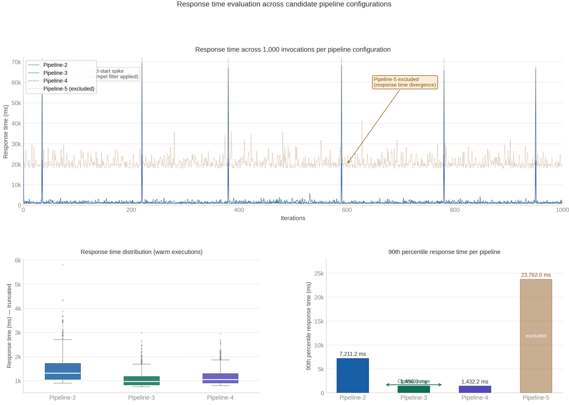
Figure 5.6: Response time distributions across the four candidate pipeline configurations (2, 3, 4, and 5 functions), illustrating the non-monotonic relationship between pipeline cardinality and end-to-end response time. The 5-function pipeline is excluded from further analysis due to response time divergence.
