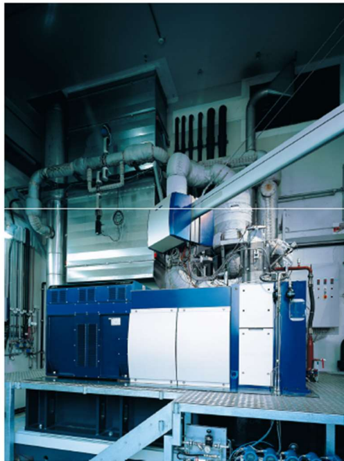
Figure 2-1. Photo of the experimental installation of the AVL FM250 single-cylinder compression-ignition engine [38]
