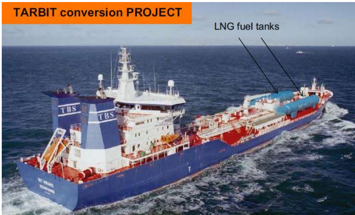
Figure 1-29. Conversion of TARBIT MT BIT VIKING for operation of its main and auxiliary engines with natural gas. The figure shows the location of LNG tanks on the deck of the ship [28-34]
