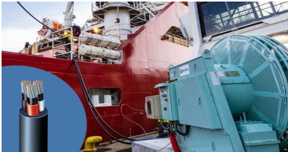
Picture 4. Shore-side Electricity Cable Reel (Source: Cavotec)
