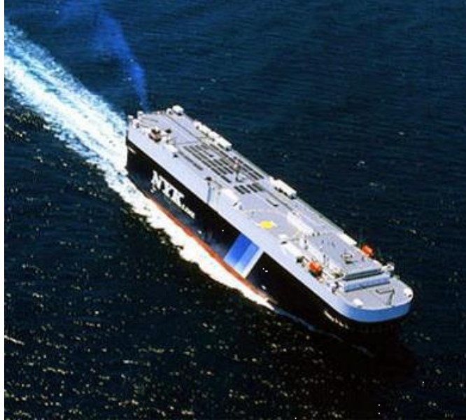
Picture 17: MV Auriga Leader with solar power array, NYK Lines (IMO, DNV, 2023)
