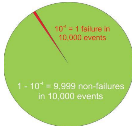
Figure 4: The imbalance between things that go right and things that go wrong (Hollnagel, et al., 2015)
