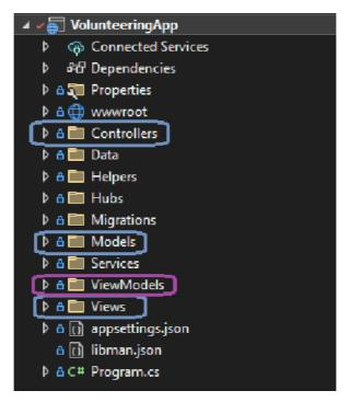
ViewModels folder contains *ViewModel* classes that are used just to render data to the views in the project and <u>do not handle any data-related operations</u> like Models do.
