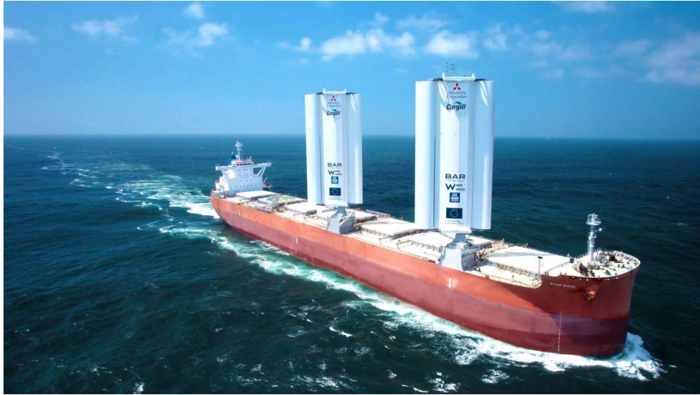
Εικόνα 9: Fixed sails (European Climate, Infrastructure and Environment Executive Agency, Αύγουστος 2023)
