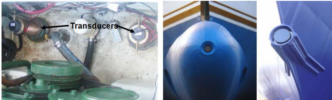
Figure 17: FL-Sonar Transducer Installations (1a. Dual EchoPilot Transducers Mounted Athwartships (left) and b. Single FarSounder Bow-Mounted Transducers (centre and right))
