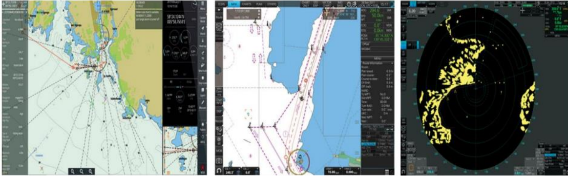
Figure 7. Different interfaces of ECDIS and Radar systems (Left to right: A Simrad ECDIS Interface, a Furuno display ECDIS Interface, a Furuno Radar Interface). Retrieved from [1], [2]
