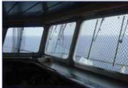
Figure 4 / Shielding of ship bridge glazing (Source: https://www.imorules.com )
