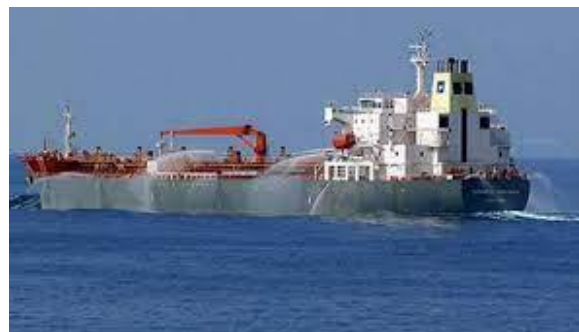
Figure 5 Water jet under pressure while sailing to prevent pirate attack. (Source https://www.sail-world.com ).
