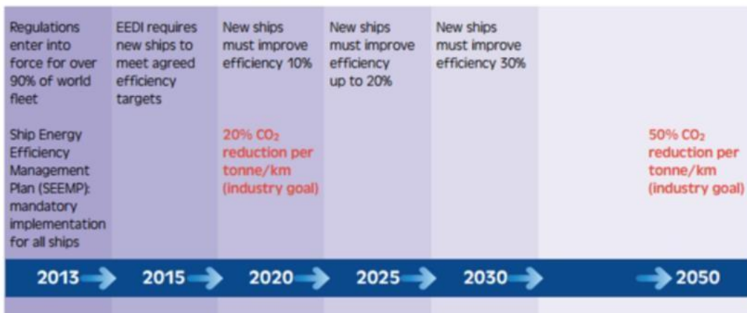
Σχήμα 4: Diagram showing the IMO's plan for ship improvements from 2013-2050 (International Chamber of Shipping)
