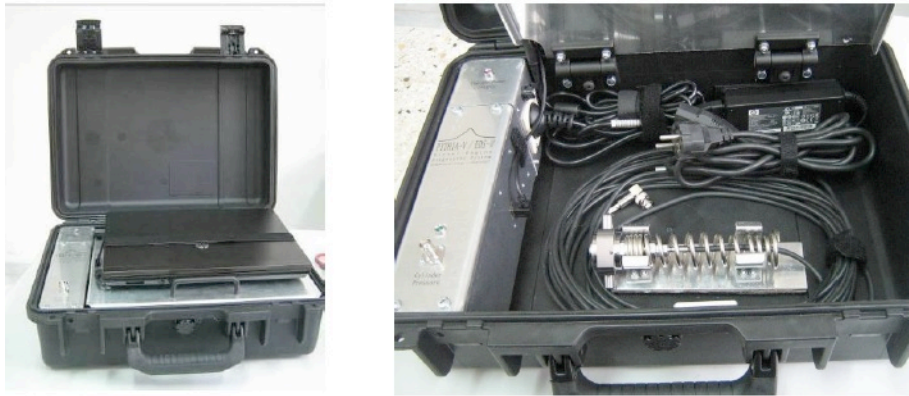
Figure 49. Portable system for taking pressure measurements of a cylinder pressure measurement E.M.P. [3]
