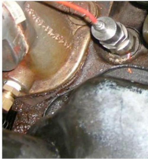
Figure 71: Photographic illustration of the position of the vibration accelerometer on the cylinder head between cylinders #1 and #2 [12]
